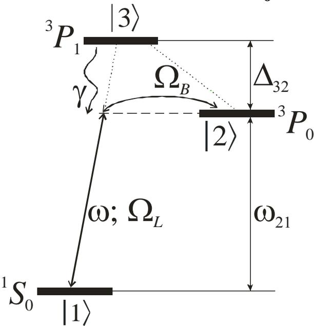
For mixing the state  $^3P_1$  with the state  $^3P_0$  we use an external static magnetic field.
