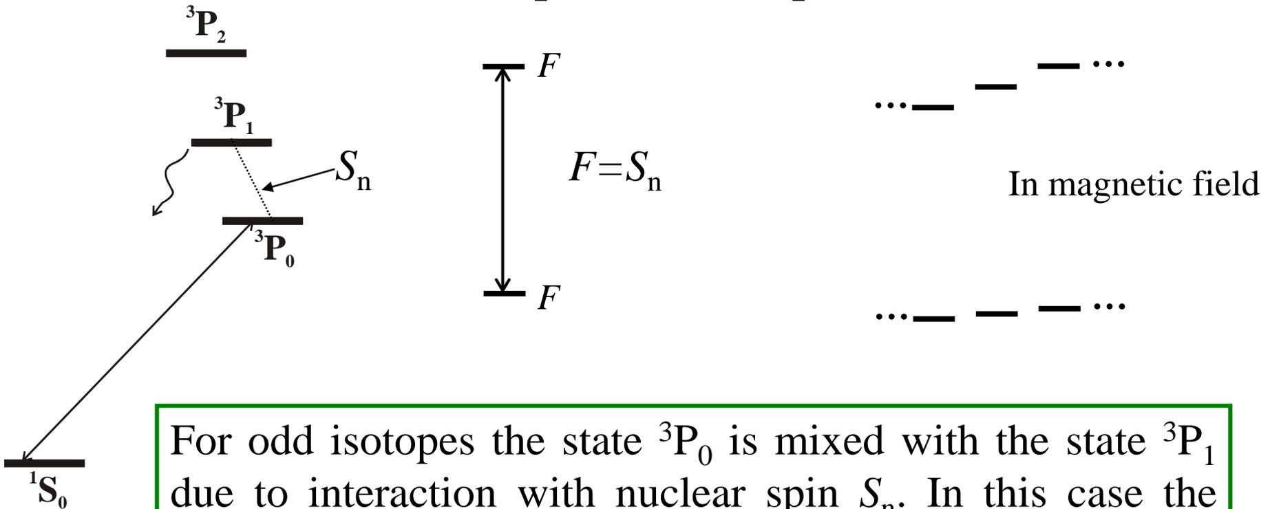
For odd isotopes the state  $^3P_0$  is mixed with the state  $^3P_1$  due to interaction with nuclear spin  $S_n$ . In this case the transition  $^1S_0 \rightarrow ^3P_0$  becomes partially resolved (natural width  $\sim$  mHz). And we can excite this transition by usual one-photon method with small intensities of probe laser. The same energy picture we have for some ion clock (e.g., for  $^{27}\text{Al}^+$ ,  $^{115}\text{In}^+$ )
